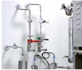
Two seals close the feedthrough according to clean-room standards: the first seal is located on the back of the CleanShut system and provides a seal between the housing and the clean room wall. The second seal is located in the inner passage of the feedthrough and seals it off. This design thus makes using additional sealants unnecessary.
