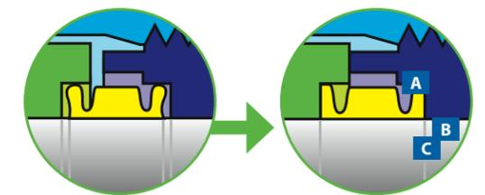
*The seal ring adapts to fit perfectly when pressed in, ensuring complete sealing and no dead space*
